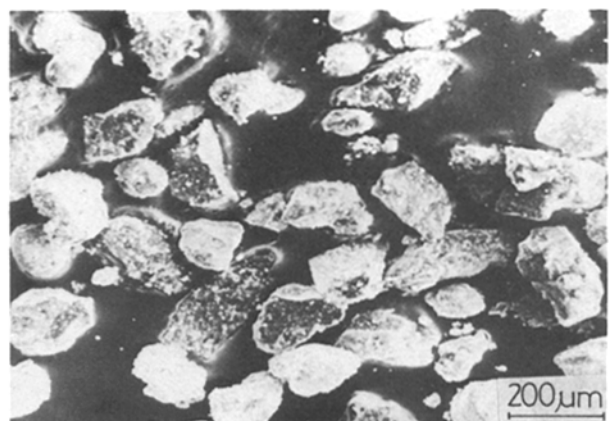
Figure 3 SEM micrograph of extracted sand showing the reduction reaction at the surface of the particles.
