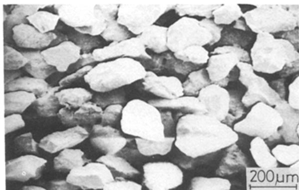
Figure 2 SEM micrograph of as-received river sand showing particle size, shape and surface.
